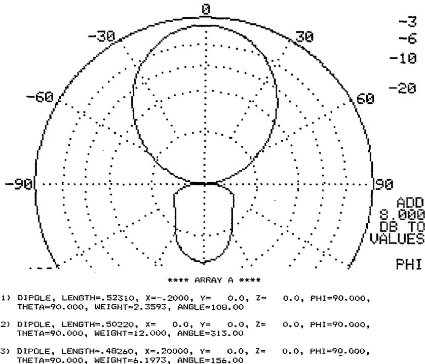
Figure 4. A Yagi antenna was analyzed by taking the phasings and weights for the elements from a MININEC calculation.
