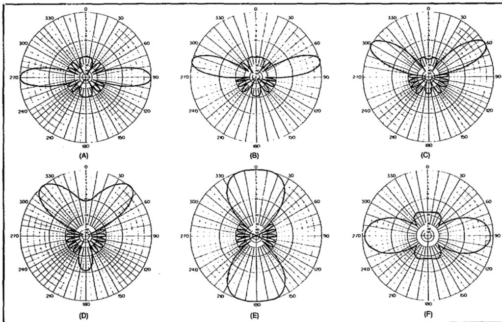
Figure 6. Chebyshev array in free space as the element phasings are changed. The elements are spaced at half wavelength intervals. At A, all the elements are in phase. Each element is given a progressive 45 degree phase shift in B. The shift is 90 degrees for C, 135 degrees for D and 180 degrees for F. At F, a poor ground causes the sidelobes to melt together.
