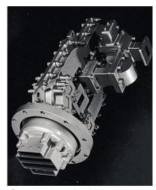
**Figure 5.** Also on the table in Figure 3 is a feedhorn comparator, comprising a number of hybrid T junctions and folded T junctions. The three ports of the comparator produce the sum and the elevation and azimuth difference patterns of the four feedhorns. This comparator is from a different antenna system.
