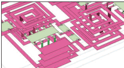
Fig. 1 A 3-D planar circuit with numerous internal ports used for mounting surface-mount devices. ▼
