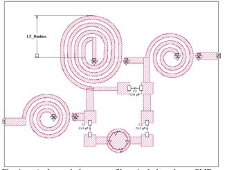
Fig. 4. A lumped low-pass filter includes three SMDs, modeled here as ideal capacitors. A more sophisticated model or measured data is easily entered as well. For highest accuracy, the reference planes in the EM analysis should be at exactly the same location as the reference planes for the SMD data.
