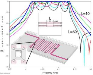
Fig. 3. The six resonator hairpin filter has two sets of perfectly calibrated ports (one set detailed, lower left) placed in the input and output coupled sections. A length, L, of coupled line (central inset) is inserted into each set of ports. As L is varied from 10 to 60 mils, step of 10 mils, new results are instantly available. The thick blue line (L=30) corresponds to the filter of Fig. 2. Notice the over 100 dB dynamic range.
