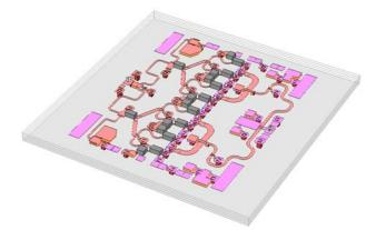
Fig. 7. For RFIC design, all transistors, capacitors, and resistors can be removed, substituting perfectly calibrated ports (small grey boxes). Now, results for design modifications are available instantly. No further EM analysis required.
